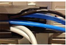
Distance from the shortest pneumatic connection to the first cable tie:
